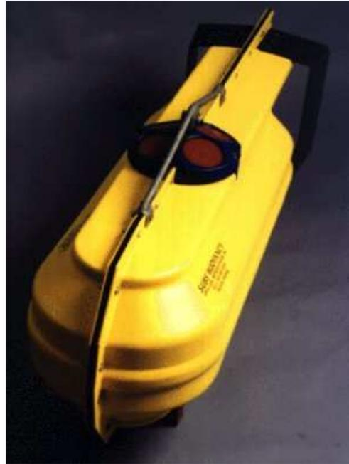
**Figure 2. ADCP meter in Subs A2 float.**
